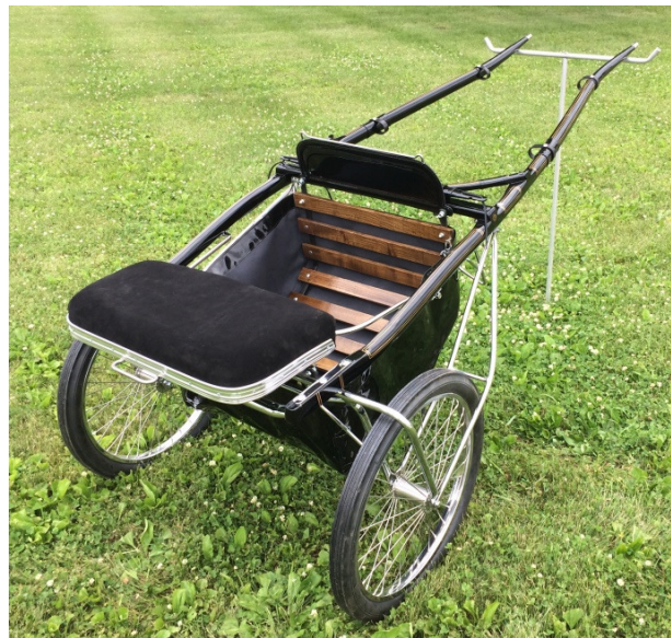
Above: Mini Pleasure Cart configured with 24” chrome wheels, chrome undercarriage, and a bench style roughout leather seat.
